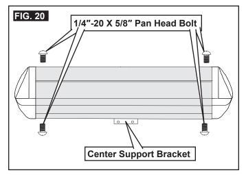
24. Attach center support bracket to slide out room wall using (2) #10-12 X 1" PHCR SS screws. See (FIG. 20) & (FIG. 21).
