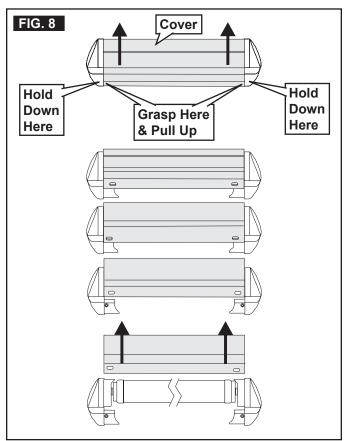
3. Carefully roll slide topper over and remove all mounting hardware if included with slide topper.
