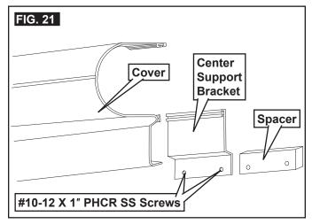
**NOTICE** ALWAYS position center support directly in middle of roller tube. Otherwise, damage to awning could occur.
